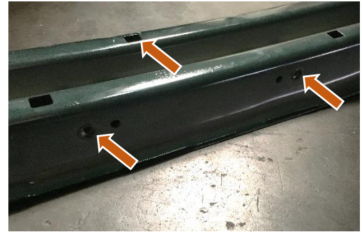
Figure 20: Front Radar and Bracket Uninstalled
