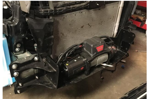
Figure 30: Winch Installed onto Winch Plate
