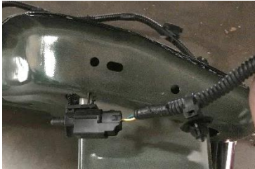
Figure 18: Temperature Sensor Removed
