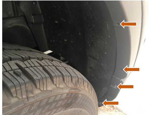
Figure 4: Torx Bolts Along Inner Wheel Well
