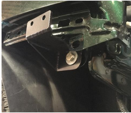
Figure 32: Outer Support Bracket Installed
