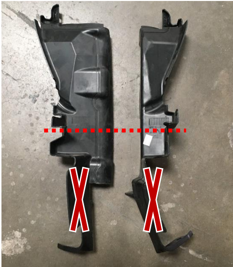
Figure 17: Radiator Air Deflector with Cut Line Shown
