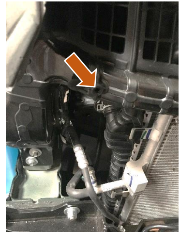
Figure 16: Upper Push Pin Location
