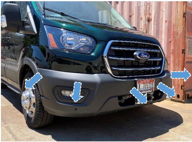
Figure 12: Factory Bumper Removal
