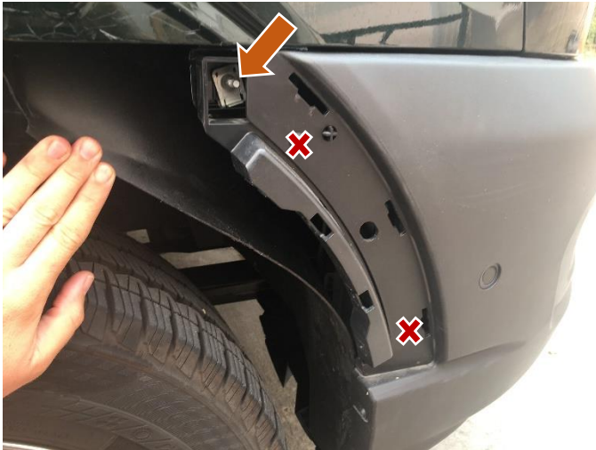
Figure 7: Bolt Accessed from Inside of the Wheel Well
