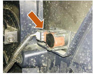
Figure 15: Parking Sensors from Backside of Bumper
