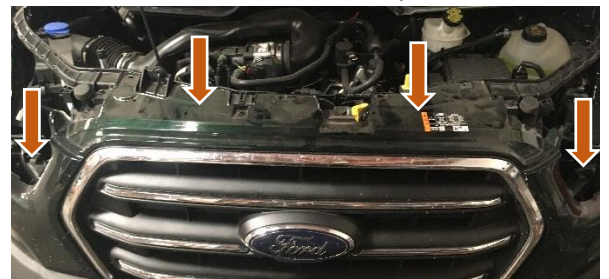
Figure 10: Locations of the Large Plastic Catches
