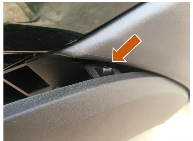
Figure 6: Fender Flare Plastic Clips Catches
