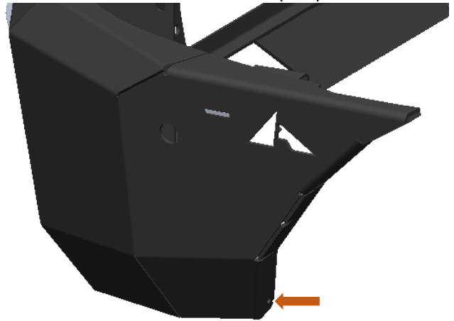
Figure 34: Attachment Point for Wheel Well Liner
