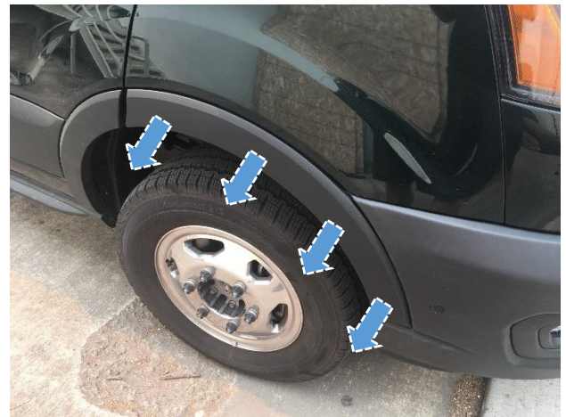
Figure 5: Fender Flare Removal
