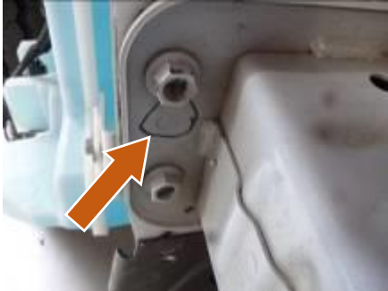
Figure 23: Example of Spot Weld (Shown from the Back)
