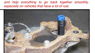
Note: We recommend spraying WD40 on all the threads and insides of bolts prior to assembling. This will lubricate
